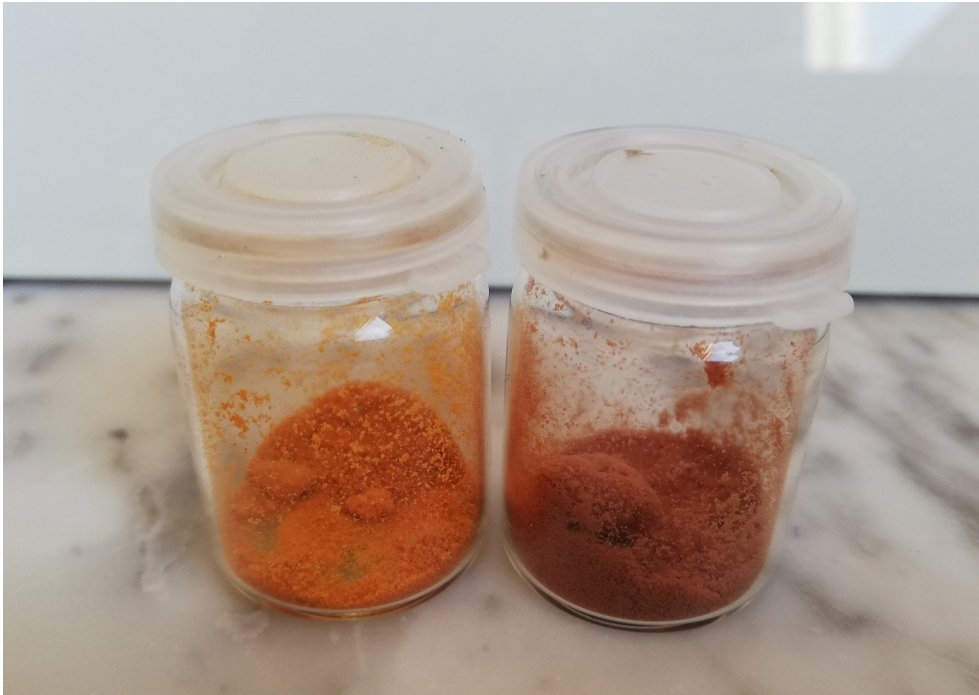
Sample of phenolic hollow beads exposed to light since 2014 (on the left) and sample stored in the dark (on the right). 06/2022.
